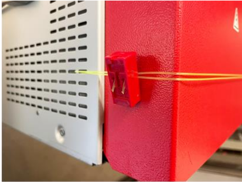
Figure 3 – Rear cover security seal example
