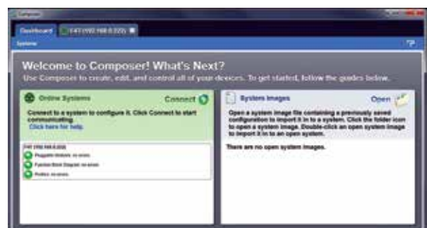
Dashboard makes it easy to connect, indicates configuration errors and allows downloading configuration files without allowing access to setup.
