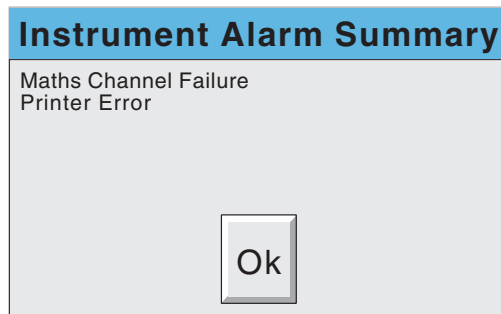
Figure 3.1.4b Typical Instrument alarm summary display
