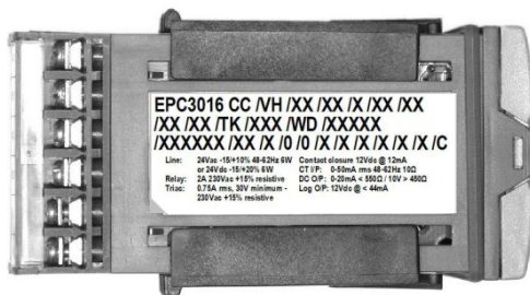
EPC3016 left hand side label showing ordering code
