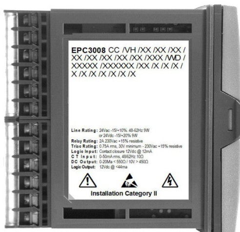
EPC3008/04 left hand side label showing ordering code
