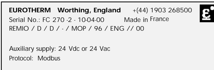
Figure 1-5 Example of REMIO identification label (corresponds to example ordering code above)
